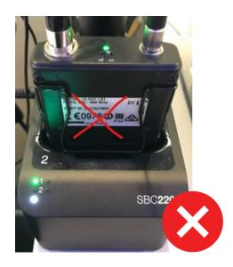
Handy Tip: Leave the microphone switched on when returning it to the charger – it will automatically turn off.
